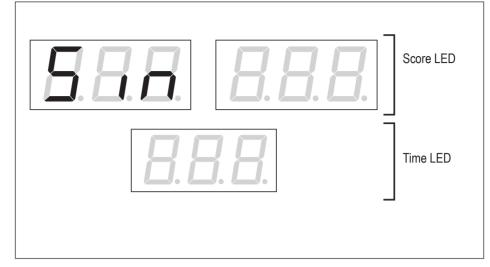
Test item selection display (Switch input test)
