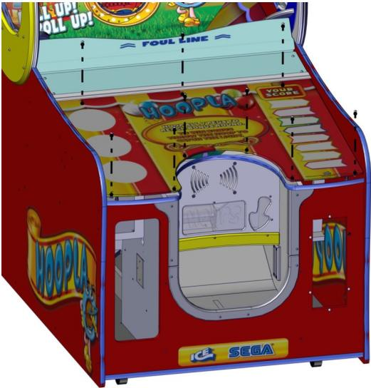
**Step 1:** Remove the control panel cover by removing the nine 5/32" Allen screws shown.
