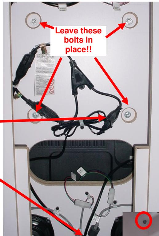
The monitor wood frame will be attached to the monitor and the wood will come out with the monitor as it is removed from cabinet.
