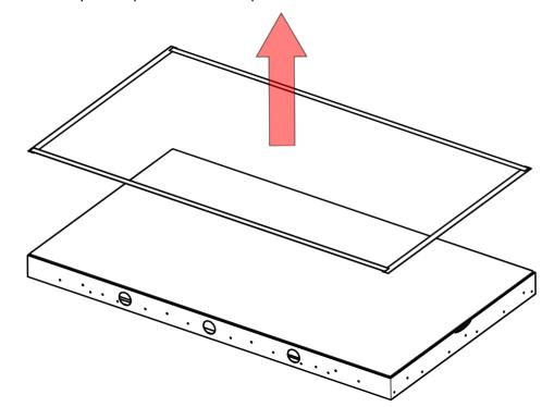
6) In a dust-free environment, remove the screen using the provided suction cups
