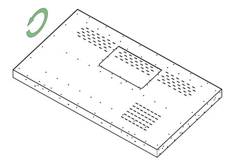
15) Screw the 28 Philipps flat head screws located on the sides near the back face of the monitor
