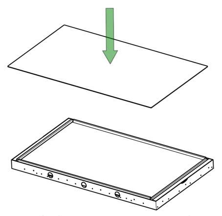
11) Clean the screen's surface using an anti-static solution and a microfiber towel
