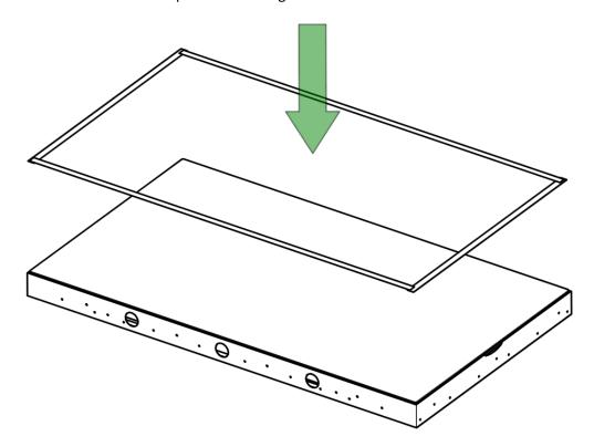
**13)** Reinstall the frame on the screen
