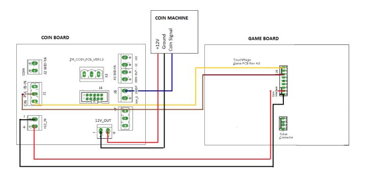
If using a mechanical roll down, use below wiring diagram.
