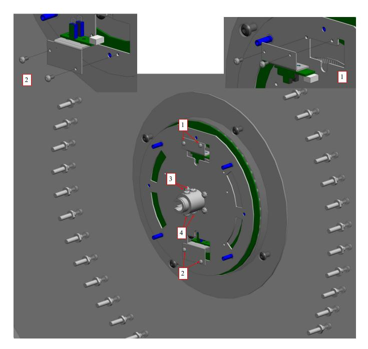
Slide the LED board out slightly and disconnect the two wire harnesses. Be sure to position the center wires so that they are straight out the shaft. Now fully slide out the ring board and
