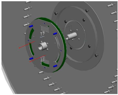
Slide the entire wheel off and put aside. When you remove the wheel assembly, be carful of any shims installed from the back as they tend to stick to the wheel
