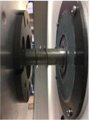
Remove one shim. Slide the metal disc back onto the clutch and spin. If you hear any grinding, replace the shim and reassembly the game.
