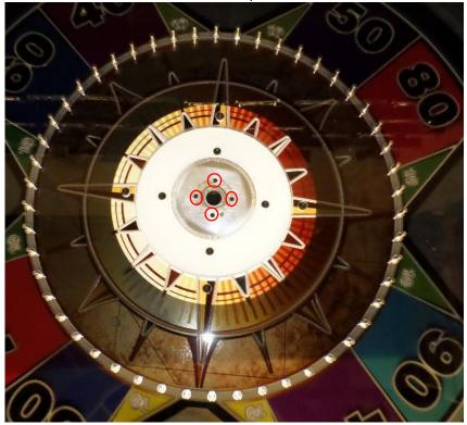
Next remove the 4 screws circled in red, these hold the clutch plate to the white inner wheel.
