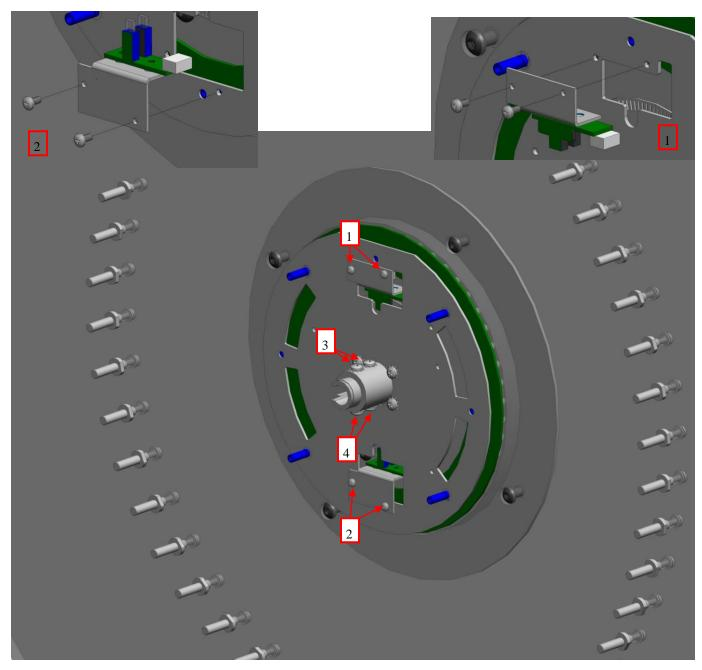
Slide the LED board out slightly and disconnect the two wire harnesses. Be sure to position the center wires so that they are straight out the shaft. Now fully slide out the ring board and put aside.
