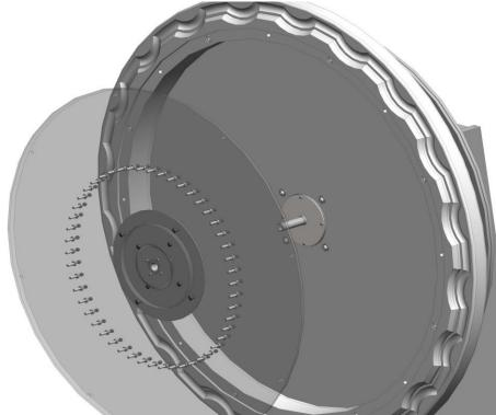
Place the wheel on a soft flat surface to avoid damage. Remove the 4 small screws circled in red holding the encoder wheel to the clutch plate. Remove the encoder wheel and screws and put aside.
