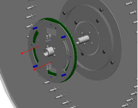
Slide the entire wheel off and put aside. When you remove the wheel assembly, be careful of any shims installed from the back as they tend to stick to the wheel assembly.
