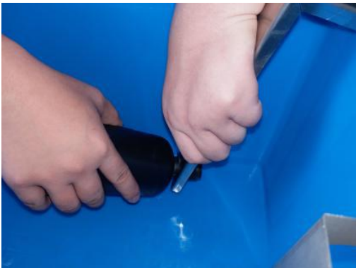
Step 5: Remove the secondary filter as shown in the following two figures.
